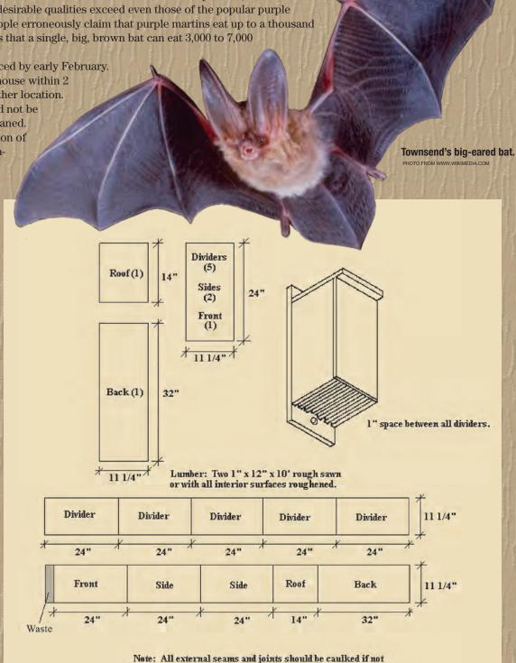
tight fitting. Divider boards are spaced I inch apart.
